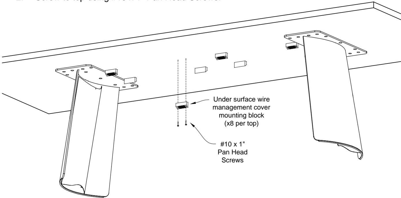
Align wire management cover so dual lock strips align and push to lock into place.
