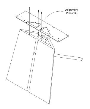
Screw base plate to base using #9 x 1 3/4" flat head screws. Remove alignment pins.
