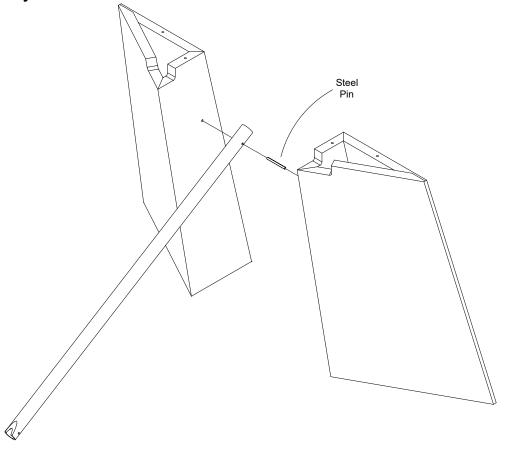
Use alignment pins (X4) to align base plate to base. Predrill holes for #9 x 1 3/4" flat head screws.
