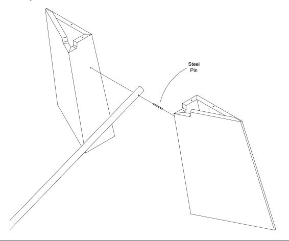
Use alignment pins (X4) to align base plate to base. Predrill holes for #9 x 1 3/4" flat head screws.
