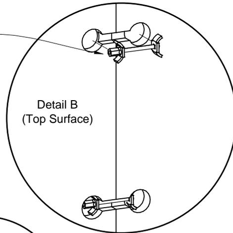
Attach drawer to subtop screwing through angle bracket into subtop using #9 x 5/8" Pan Head Screws
