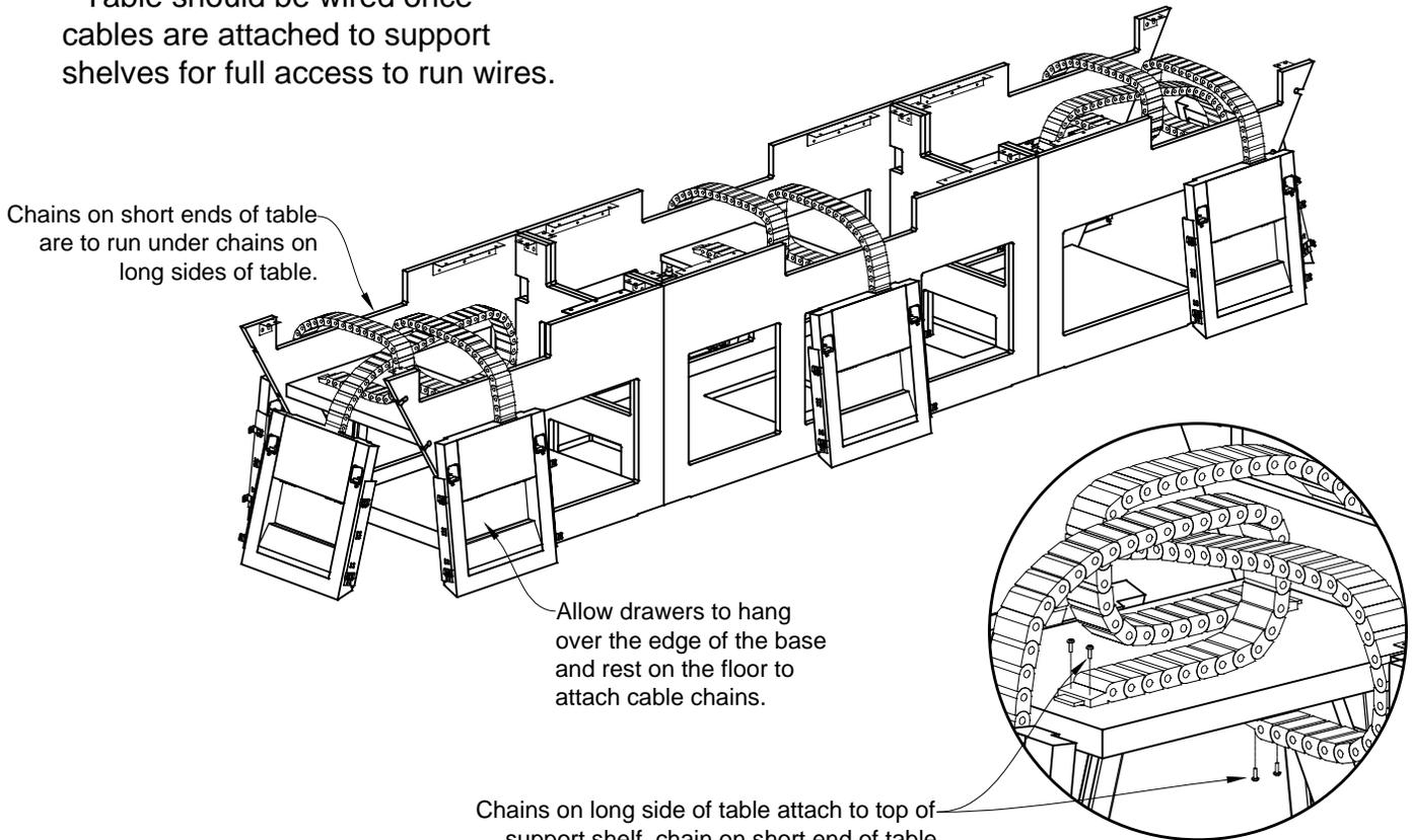
Chains on short ends of table are to run under chains on long sides of table.
