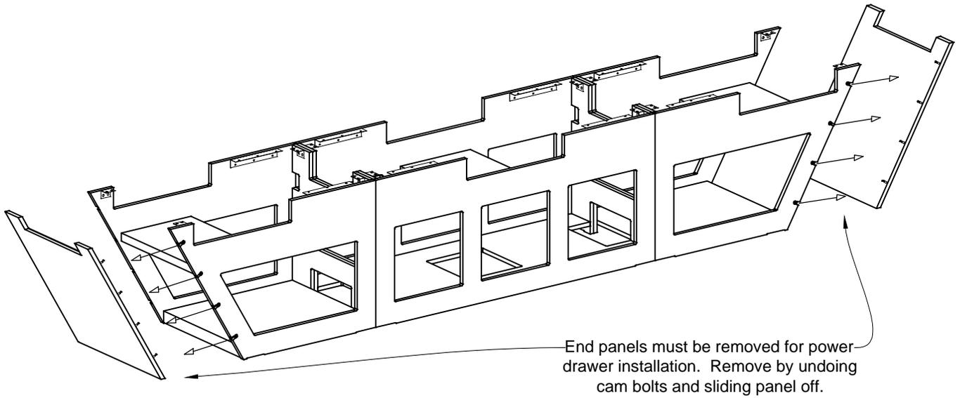
End panels must be removed for power drawer installation. Remove by undoing cam bolts and sliding panel off.
