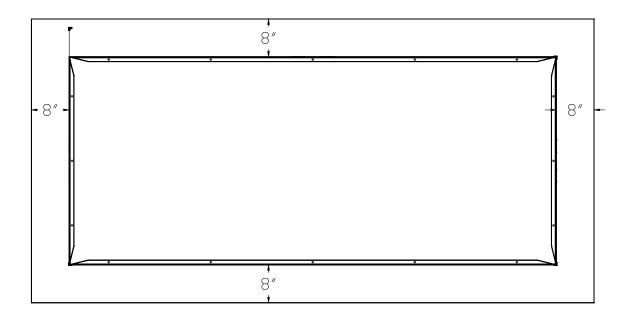
\* Screw power apron to top using #9 x  $\frac{5}{8}$ " pan head screws.
